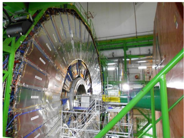
The Compact Muon Solenoid (CMS) is a general-purpose detector at the Large Hadron Collider (LHC). It is designed to investigate a wide range of physics, including the search for the Higgs boson, extra dimensions, and particles that could make up dark matter
