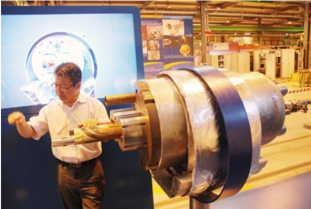
Magnets surrounding the beam tube
